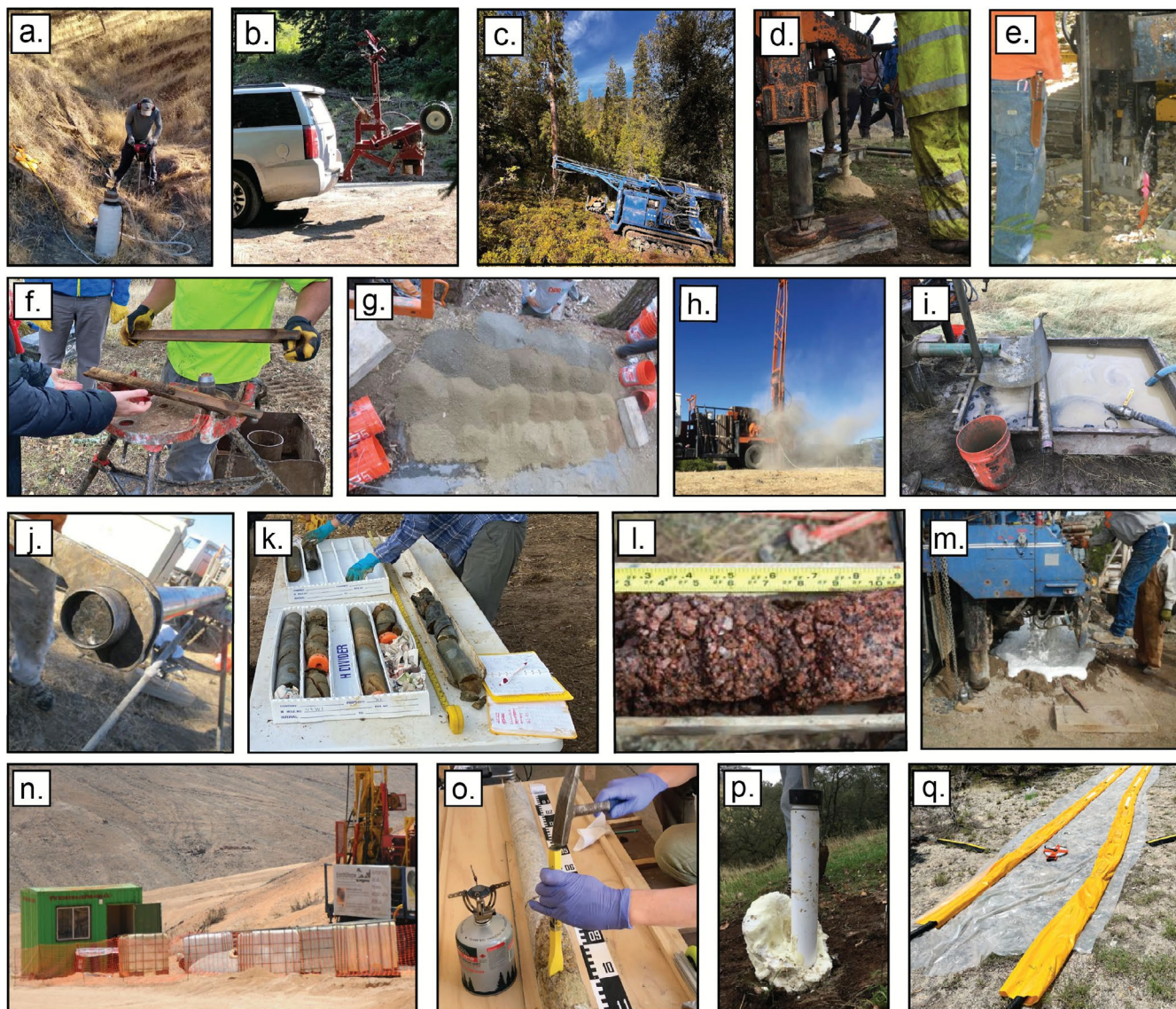
FIGURE 1 | Drilling within the critical zone photoseries: (a) Portable hand held drill with water tank, (b) portable drill that can allow for greater access to rugged terrain, (c) track-mounted drill rig navigating steep terrain with dense vegetation, (d) dry auger starting borehole and bringing cuttings to the surface, (e) drill pipe connected to subsurface for standard penetration testing, (f) recovered core from standard penetration test, (g) arranged cuttings samples by depth to show lithologic colour variability, (h) drilling without water can generate large amounts of dust, which requires personal protective equipment, (i) recycled drilling fluid and mesh to capture coarse fraction cuttings, (j) end of core barrel, the ‘shoe’ (bottom section of each core run), (k) example station for onsite rock core characterisation with PVC core carrier and core boxes, (l) example of core with highly weathered interval, (m) drill fluid additives such as foaming agents help flush drill cuttings to the surface, improve borehole stability, and reduce equipment wear, (n) temporary structure (green) provides a controlled workspace for onsite core characterisation and subsampling, (o) subsampling core interior with hammer and chisel, (p) polyurethane foam used to fill borehole casing annulus, (q) specialised sleeve with sensors and ports for vadose zone monitoring. Photographs by authors.
